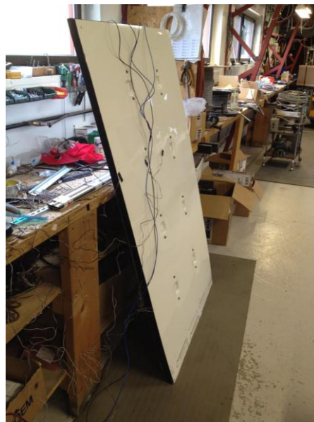
Figure 27. Picture of prototype wall. Two aluminum sheets are screwed together holding 8 TE modules in between them at each dent. The sheets are separated with insulation to prevent heat transfer between the hot and the cold side.
