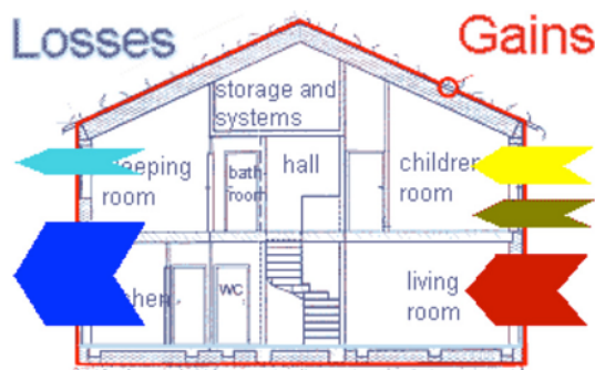
Figure 3.12: Heat losses and heat gains (Losses: transfer and ventilation losses; Gains: solar radiation, internal heat sources and persons inside the building) (Feist 2006f)
