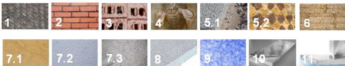
Figure 3.2: Building materials (1 - Concrete; 2 - Solid brick; 3 - Hollow brick; 4 - Wood; 5.1 - Porous concrete; 5.2 - Porous bricks; 6 - Straw; 7.1 - Mineral wool; 7.2 - Polystyrene; 7.3 - Cellulose; 8 - Highly insulation material (Heat conductivity 0.025 W/mK); 9 - Nonporous; 10,11 - Vacuum insulation)
